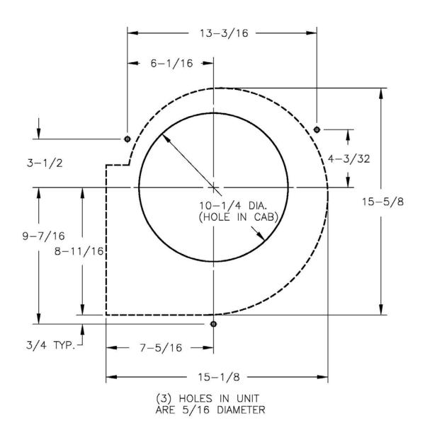
TEMPLATE FOR MOUNTING HOLE LOCATIONS AND INTAKE HOLE OPENING FOR MODEL "OE" ELEVATOR CAB EXHAUST UNIT
